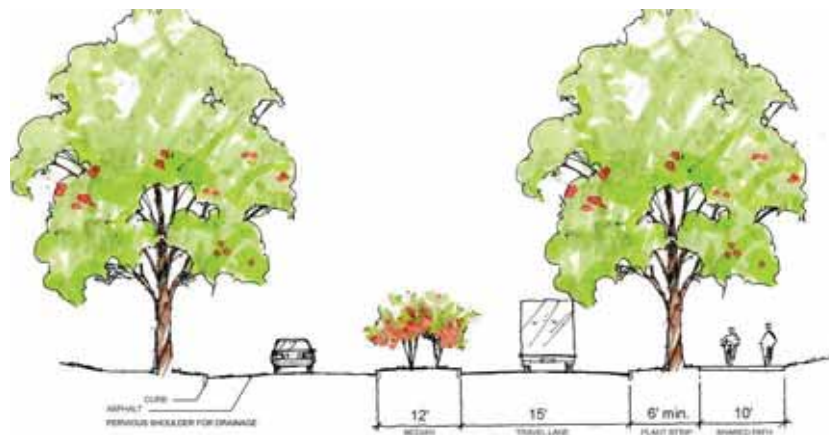
Typical cross-section of gateway entrance corridor (two lane example) showing landscaping at street and in a median (where possible) with a pedestrian/bicycle access trail or sidewalk. Shoulders of road could include natural swales or use pervious surfaces to manage stormwater runoff.
